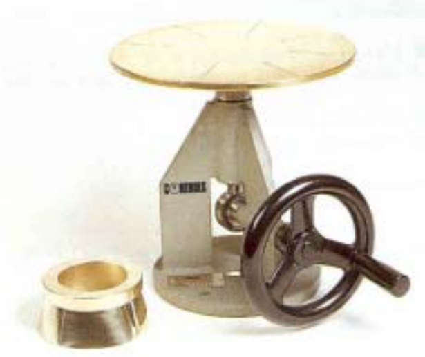
a) Flow Test Equipment
