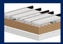
Beam centres may be closed up by re-orientating infill block, as indicated on the contract layout drawings.
