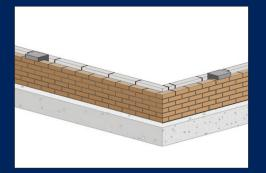
Air bricks installed. Requirement for 1500mm² of free air flow per metre run of wall, or 500mm² per square metre of floor area, whichever is greater.
