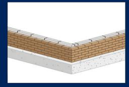
Walls taken up to DPC level. Top soil and vegetable matter removed. Void to be provided to underside of floor.
