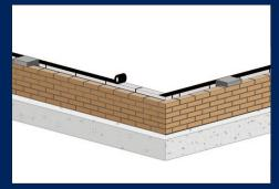
DPC to be provided under bearing ends of floor beams. The bearings for the beams should be clean, level and free from debris. The mortar in the masonry must be cured and have sufficient strength to support the floor.
