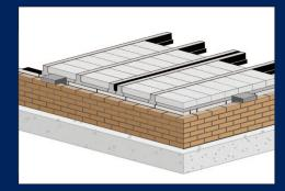
Beams may be doubled up if required by the contract layout drawing. The space between the beams above the flanges must be filled with in situ concrete of minimum compressive strength 30N/mm<sup>2</sup> with 10mm sized aggregate.
