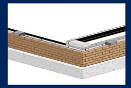
First beam is positioned using contract layout drawings supplied by CEMEX Floors technical office. Split course blocks to be provided under infill blocks where built into support wall.
