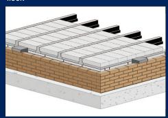
Infill blocks installed to whole of floor area. On completion a sand/cement (4:1) slurry grout to be applied to whole of floor area. Floor does not form a stable working platform until this has been carried out.
