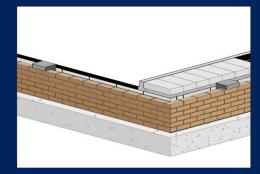
All infill blocks to be fully bedded onto split course blocks. Split course to be bedded onto support wall below.
