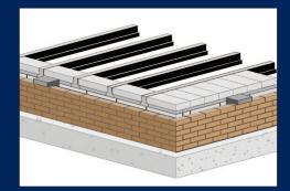
The floor may be installed using the infill block as spacers between the ends of the floor beams. Spacings will be indicated on contract layout drawings supplied by CEMEX Floors technical office.
